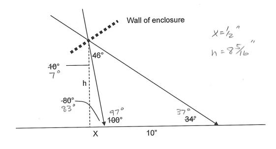
a) Specify the sun-high and sun-low lines; here, they are lines with elevations of 80° and 34°, respectively.
