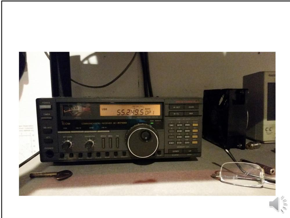
The receiver is an ICOM 7000 general coverage HF/VHF/UHF receiver, set to receive Single Sideband signals. It is fed with 50-Ohm, RG8U cable from the antenna.
