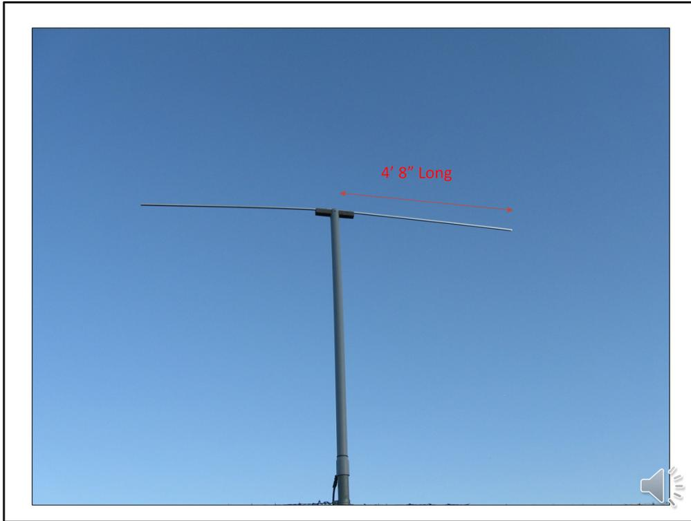
The antenna used for the Meteor Reflections Monitoring Telescope is a horizontal, half-wave dipole. **+PRESS** Each dipole of the antenna is 4' 8" long. The dipole is resonate at 55.250 MHz.
